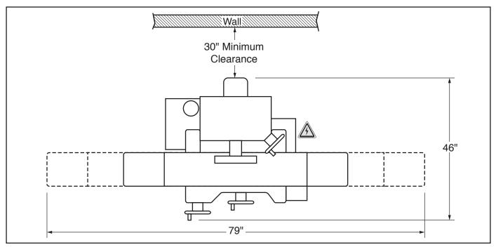
Figure 10. Minimum working clearances.
